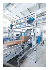
or if a package is too large to be conveyed, it's better to route that package differently from the start. Image-based readers and dimensioning sensors, placed at key points near receiving, allow for smoother workflows.
