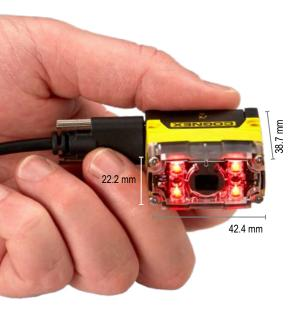
Cognex barcode readers are optimized with patented algorithms to ensure industry-leading 99.9% read rates of 1D and 2D symbologies in the most challenging barcode reading applications.
